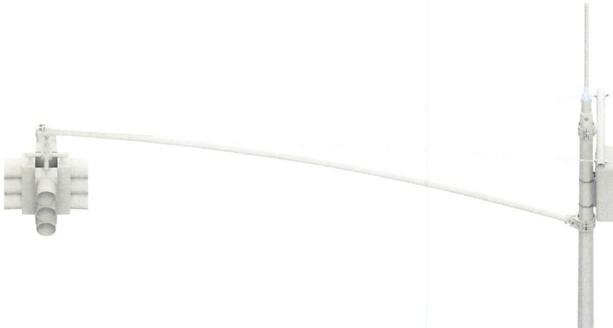
Figure 2-4: Type M-2 Traffic Signal Pole
