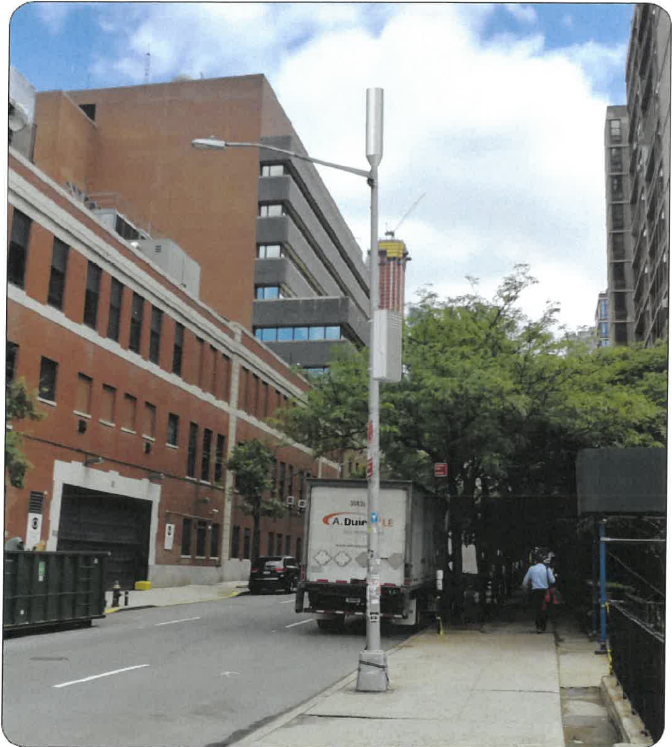
Figure 2 – Photosimulation of larger shroud with multi-technology antenna solution.
