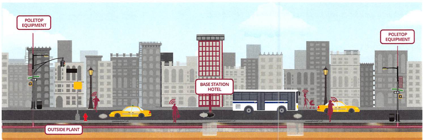
Image 2: Transit Wireless proposed network architecture for poletop
